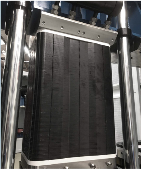
New generation Proton Exchange Membrane (PEM) electrolyser module enabling larger-scale hydrogen plans (Gigastack project – BEIS, ITM Power, Ørsted, Element Energy)
